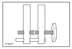
This will prevent the cooling system from filling which may lead to water being injected into and filling the exhaust system. Without the engine running there isn't any exhaust pressure to carry the water out the exhaust outlet.
