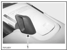
GTX RFI MODELS 1. Shift lever in reverse position
