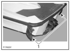
1. Side vane turns following steering movement
