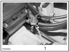
GTX RFI MODELS 1. Hose pincher
