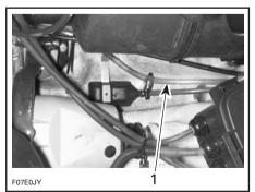
1. Engine cylinder drain hose
