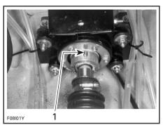
1. Grease seal carrier of mid bearing
