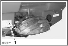
GTX RFI MODELS 1. Reverse gate in middle position
