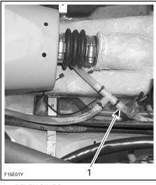
787 RFI ENGINES 1. Engine drain hose
