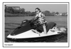
Turning the handlebar pivots the jet pump nozzle which controls the watercraft direction. Turning the handlebar to the right will turn the watercraft to the right and inversely. The throttle should be applied to turn the watercraft.
