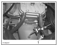
717 AND 787 RFI ENGINES 1. Engine water outlet hose
