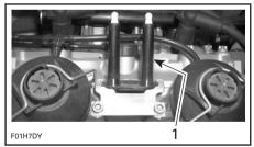
RX, RX DI AND GTX MODELS 1. Grounding device
