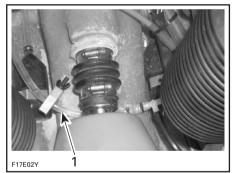
GTI MODELS (717 ENGINES) 1. Engine drain hose
