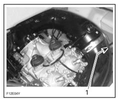
*947 CARBURETOR-EQUIPPED ENGINES* 1. Tuned pipe bleed hose
